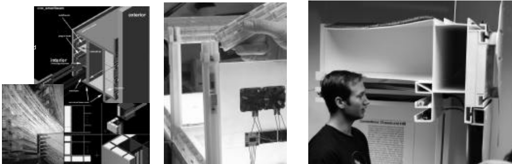
Fig. 1. House_n chassis system: axonometric, scale model with embedded networking, and full scale study model (House_n study).
