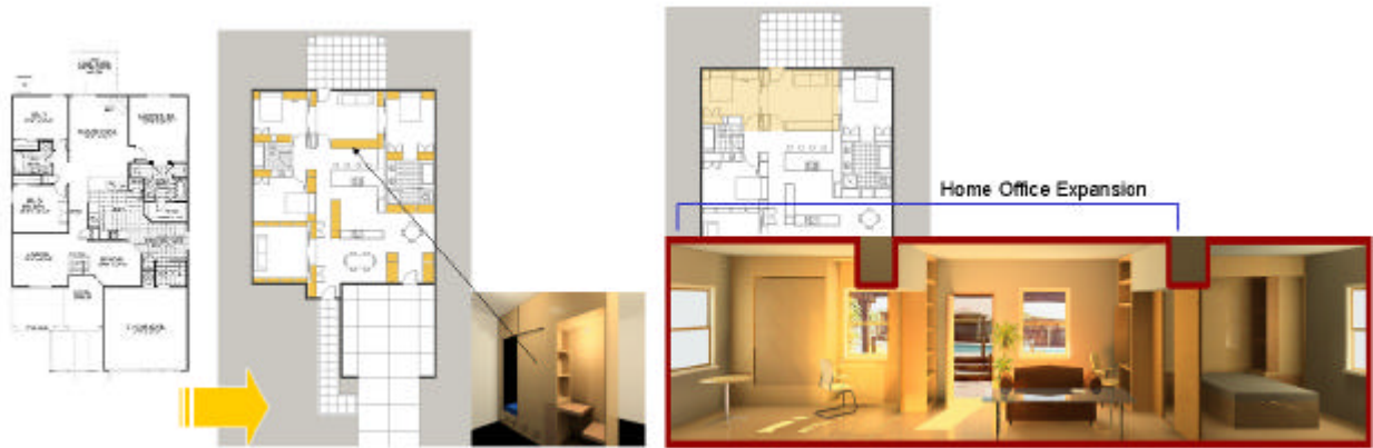
Fig. 2. The floor plan of a conventional builders house has been duplicated using interior cabinet-like components (House_n study).
