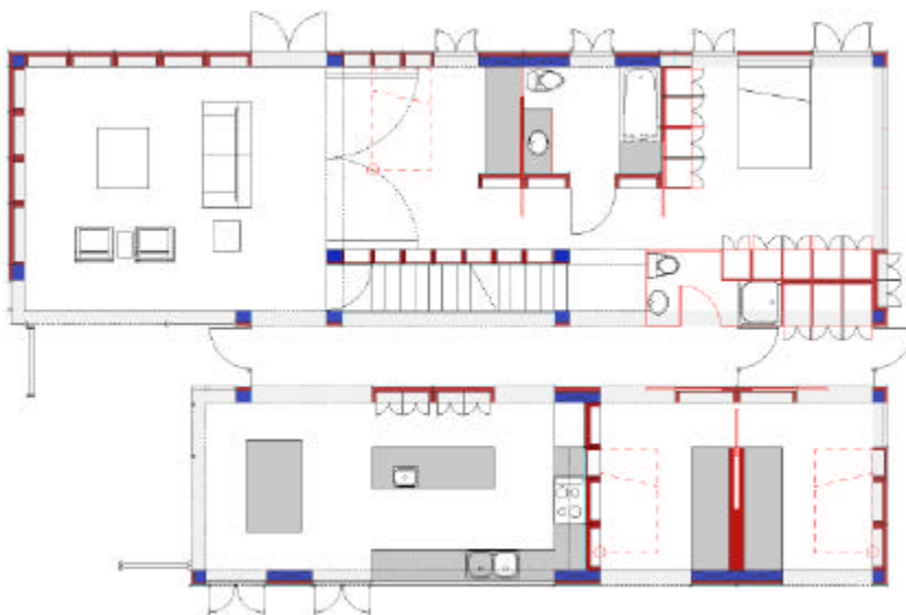
Fig. 3. Prototype plan with chassis/infill components (House_n study).
