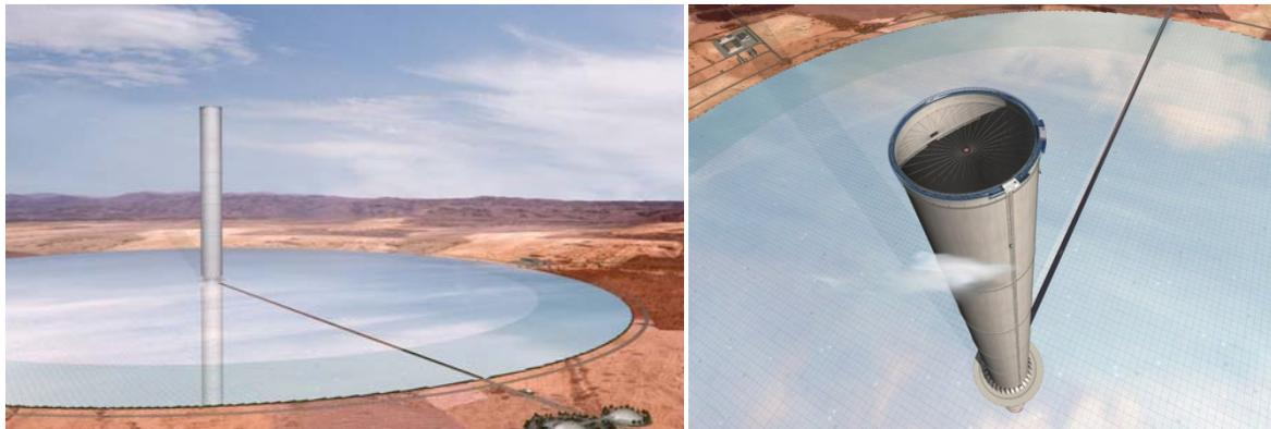
Solar Updraft Towers, mainly suitable for large-scale energy production in units of 100 MW or more, can be erected by local labor force and to a high degree with locally available materials.
