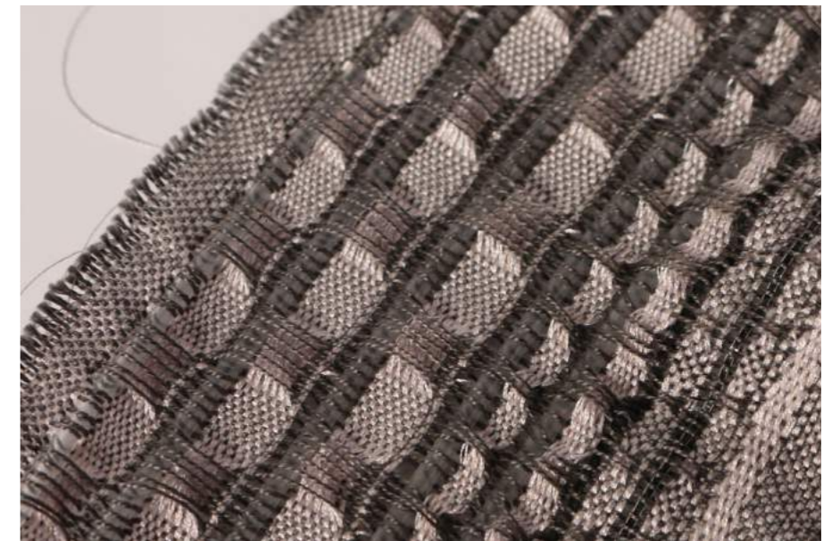
Offset networks of conductive fibers and silicone tubing in different spacing. Calibration of embedded versus exposed nature of the silicone tube.
