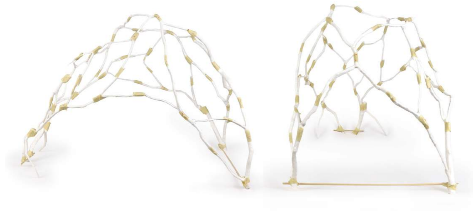
Early prototypes using manual assemblies and an additive approach with a non-predetermined topology. The elements were 3D printed scans of the inventory branches.
