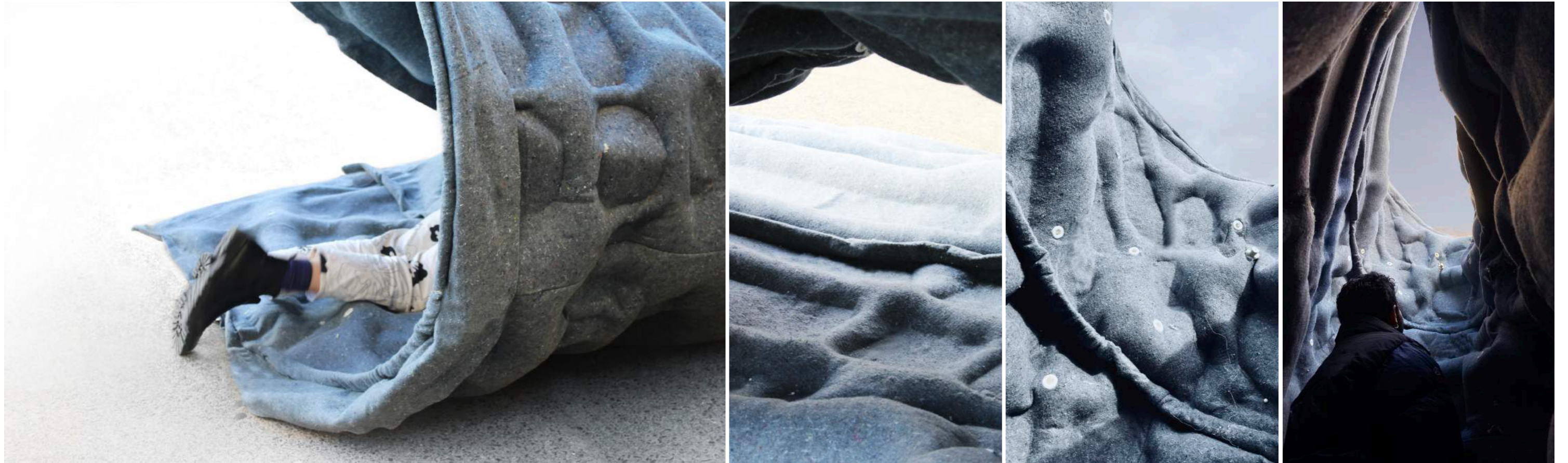
Details from the inflated foam-felt surfaces. The white circular elements were plugs from which the spray foam straw was inserted and foamed.
