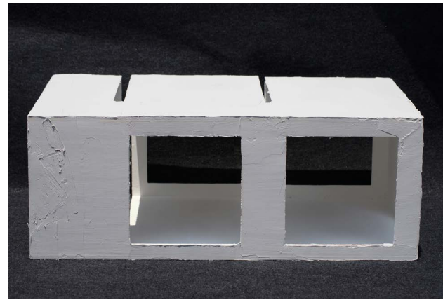
Process maquette, first application of microcement, before sanding
