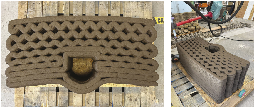
Figure 7 Raw earth walls can be 3D printed to climate-specific geometric configurations of thermal mass and insulative voids. Here a 1 \times 0.5 \times 0.5 wall section demonstrates the functional layout of material for thermal performance in Santa Barbara, California, as well as integrated formwork for a reinforced concrete column.
