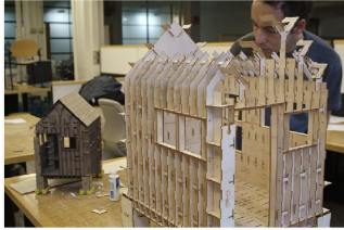
Discovery of scalable assembly; smaller model constructed of .09mm thick sheet goods & larger model constructed of 3mm thick sheet goods
