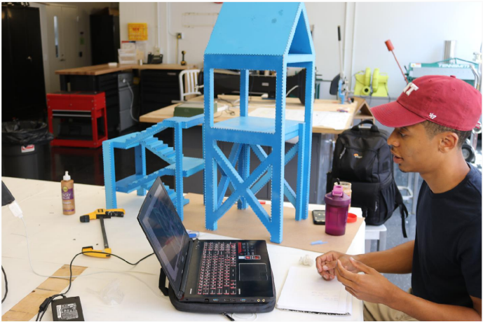
Assembled Plate Forming model with finger joints by a visiting student from Tuskegee University (2018)
